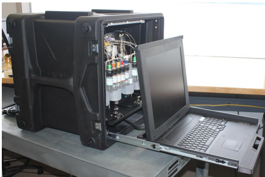
Figure 4: FloPro-Tracker with pull-out screen, keyboard and pointing device
