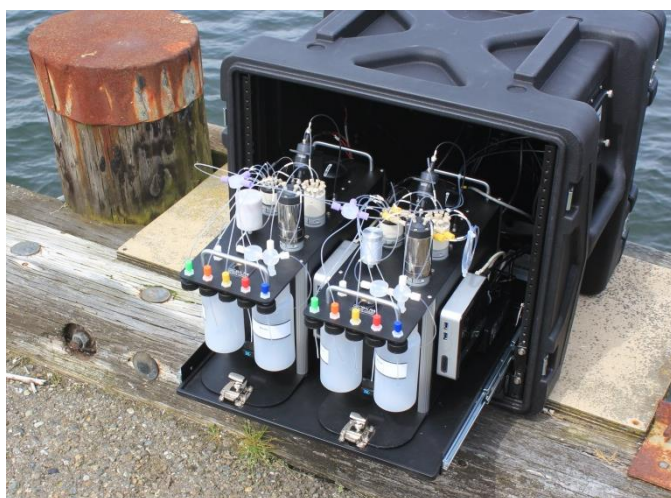
Figure 2: FloPro Analyzers installed in the FloPro-Tracker 19" rack
