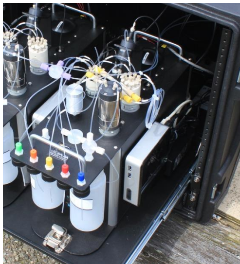
Figure 3: FloPro equipped with milliGAT pump, multi position selection valve, heated reactor, cadmium reactor (for NO 3 determination), spectrometer and flow cell, GPS and miniaturized NUC computer
