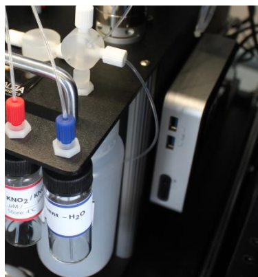
Figure 6: Intel NUC computer mounted on FloPro
