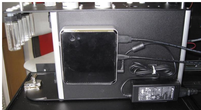
Figure 15: NUC computer and power supply mounted on the side of the FloPro analyzer
